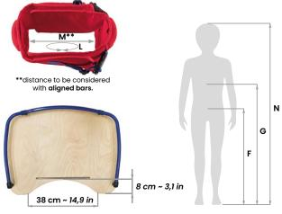
Make sure that measures F and G indicated in the figure do not exceed the suggested range indicated for the supports.
