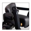
**Built-in up/down switch** Raise and lower the TRAM using the single button built into the right steering handle.
